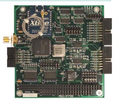
Slave relationships. Modules remain synchronized without use of master/server configurations for rapid synchronization times and fast cold start times. It can also be programmed for NonBeacon mode as either a Coordinator or End Device. The Coordinator mode can be configured to use either direct or indirect transmissions. It will also support Unicast or Broadcast communications.
