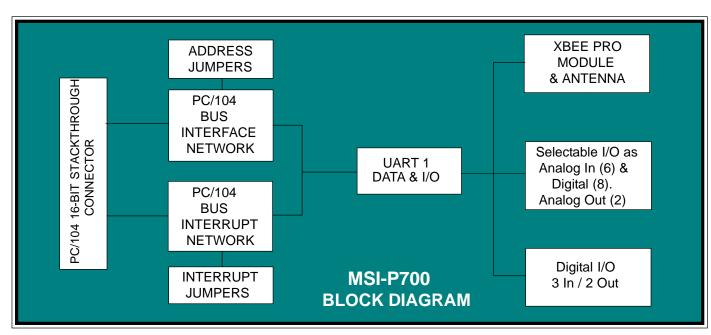
from 1200 to 115.200 bits/s. Automatic hardware RTS and CTS flow control is used to prevent overflow of the local receiver and remote receiver FIFOs. The card I/O address is jumper selectable for COM1 thru COM4 with an optional 16-bit offset address. Interrupts are jumper selectable for IRQ3 thru IRQ5 and IRQ9 thru IRQ15.
